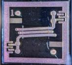
Single piece of onsilicon thin film solenoid inductor (3.5 mm x 3.5 mm) placed on a foreign silicon substrate after successfully completed µTP processing.
